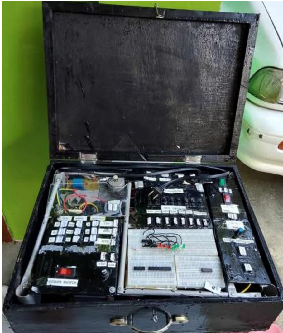
Figure 2. Picture of the Modified Electronic and Digital IC Trainer with a carrying case.
